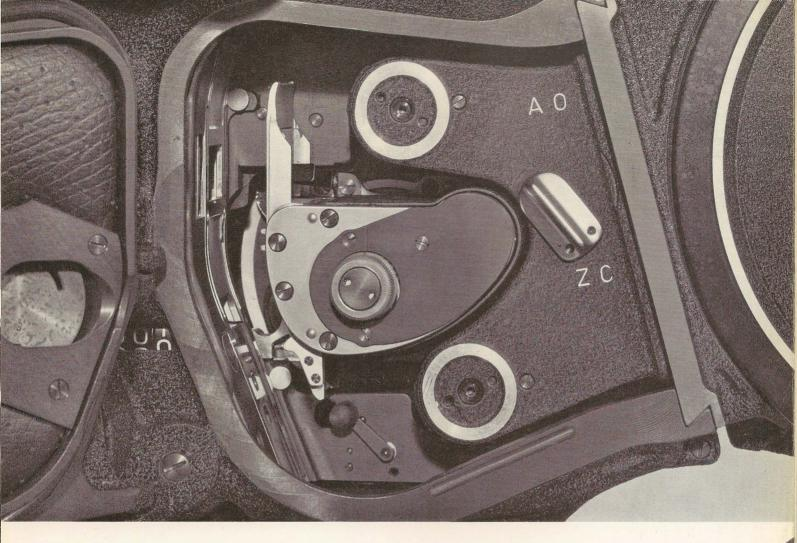
The claw mechanism can be pushed back for quick film threading and easy cleaning of the film gate
